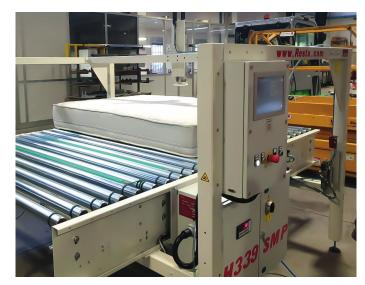
Mattress dimensional control station, equipped with a roller conveyor, that can be used independently or included into a production line.
