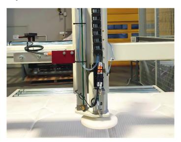
Probe for load-bearing capacity testing (automatic multi-zone detection on request).
