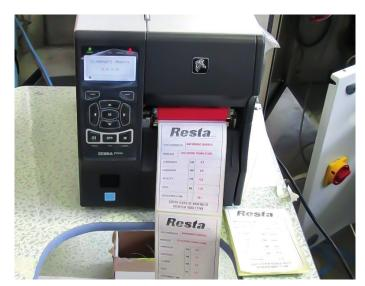
C ustomizable printer, ideal for inserting the data detected by the H339 SMP into pre-defined fields, on adhesive labels or cardboard.
