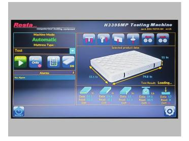
Touch screen control panel where all the functions and values detected during the objective and comparative checks are highlighted.
